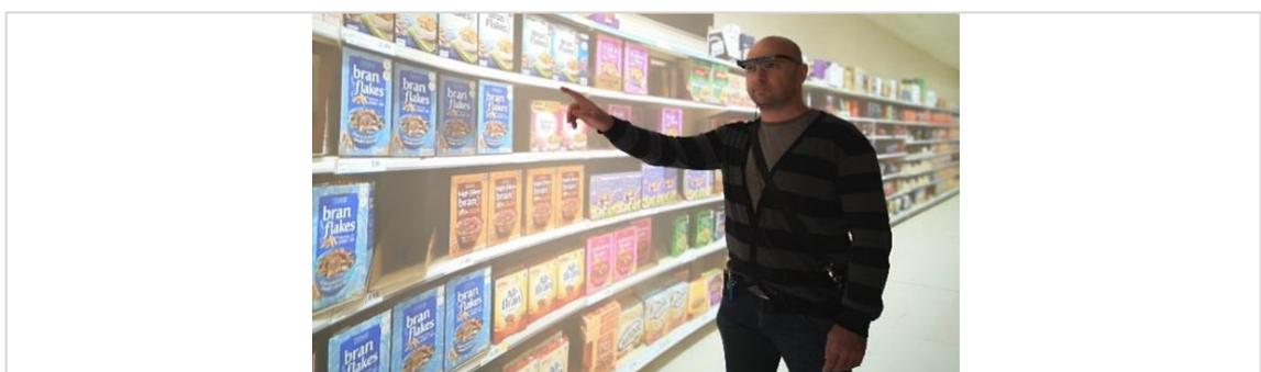
Figure 13: PEL-3 – Cylindrical media rear projected onto the PEL screen to replicate real-life shopping aisle scenario for user testing.
