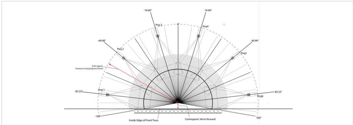
Figure 10: Throw calculations: projector locations and edge blending calculations.
