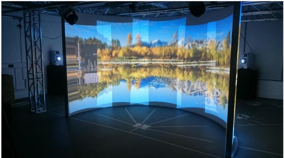
Figure 11: PEL-3 – Truss structure with custom cylindrical screen being rear projected.
