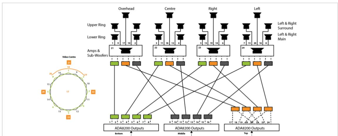
Figure 15: PEL-3 – Audio system schematic.
