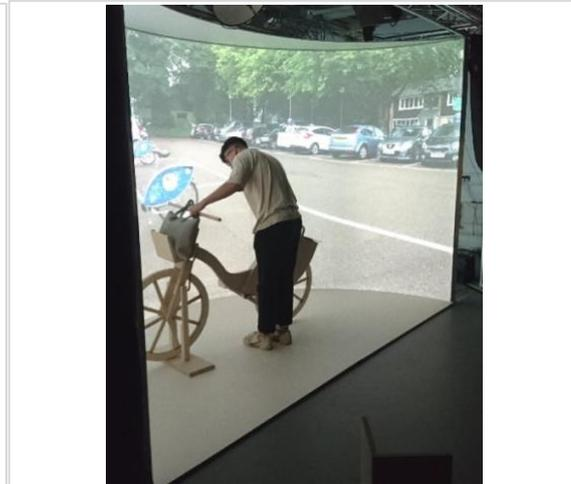
Figure 18: Next Bike usability testing: Eye-tracking glasses were used to study behavior in the PEL-3.
