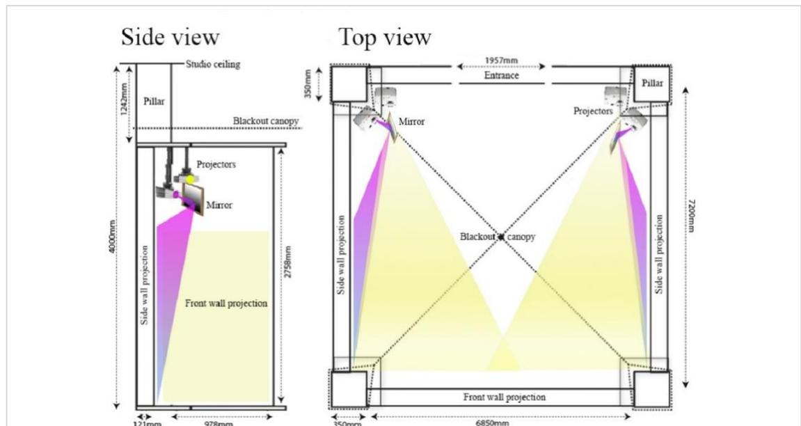
Figure 4: Projection paths using ceiling mounted first-surface mirrors and projectors.
