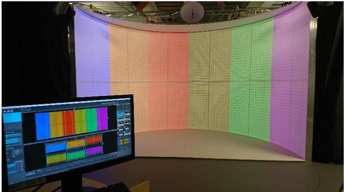
Figure 12: Mad Mapper VJ application showing surface template mapping.
