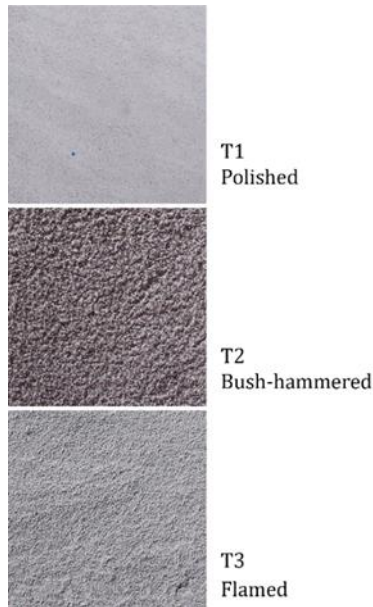
Figure 2: Tactile samples of Pietra Serena textures: (T1) Polished, (T2) Bush-hammered, and (T3) Flamed
