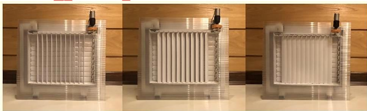
Figure 11. Small-scale prototype of the designed movable façade in three states: open, semi-open, and closed. Source: Authors.
