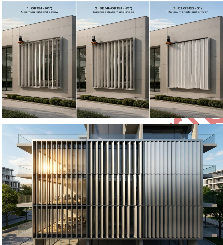
Figure 12. Different applications of the designed movable façade on building elevations through dimensional variation, according to the preferences of the architect or client. Source: Authors.
