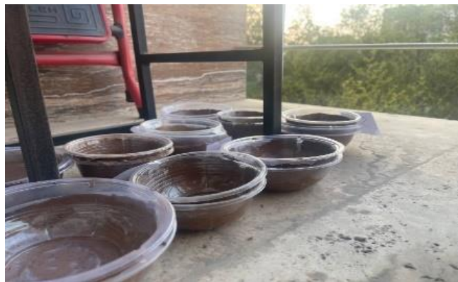
Figure 9: Drying the Composite in the Mold. (Source: Author)
