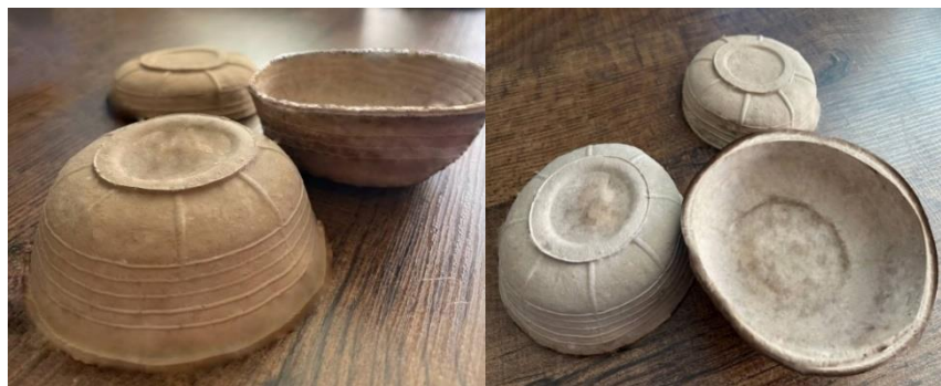
Figure 10: Containers Produced by Molding; Bowls Released from the Mold (Source: Author)
