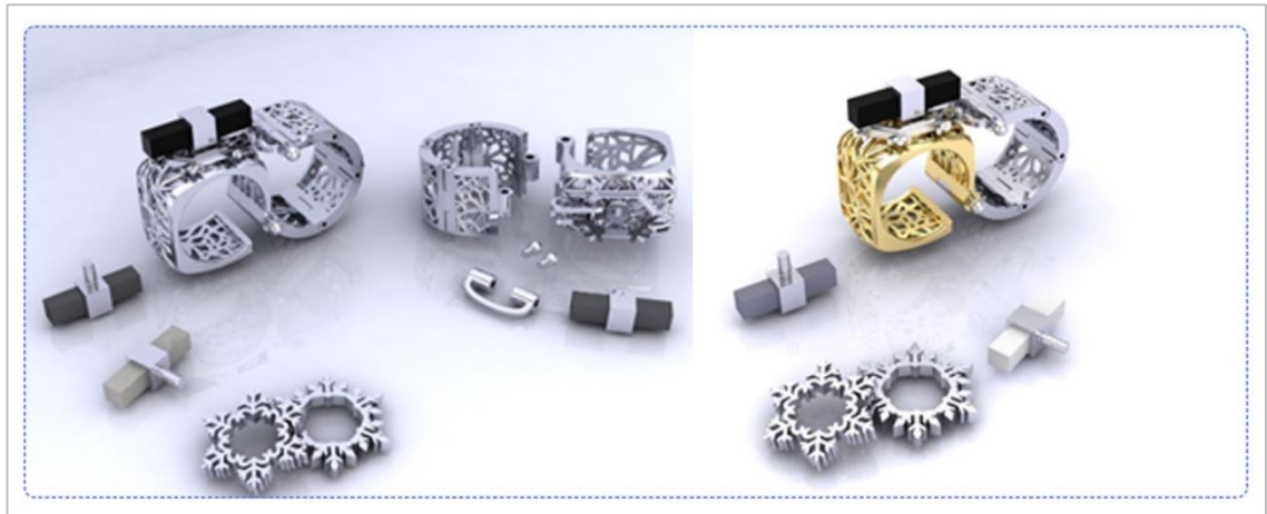
Figure 11: Exploded view of the final design detailing the 7 essential components and pin connections
