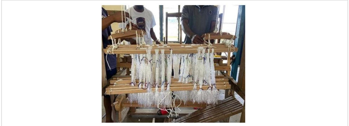
Figure 7: Connecting and adjusting the shedding mechanism of the 8-shaft broadloom.
