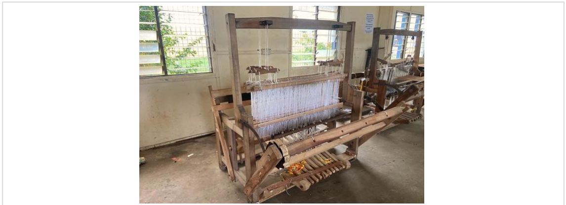
Figure 8: The Retrofitted 8-shaft broadloom.
