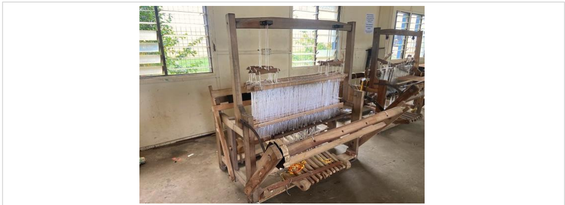
Figure 8: The Retrofitted 8-shaft broadloom.
