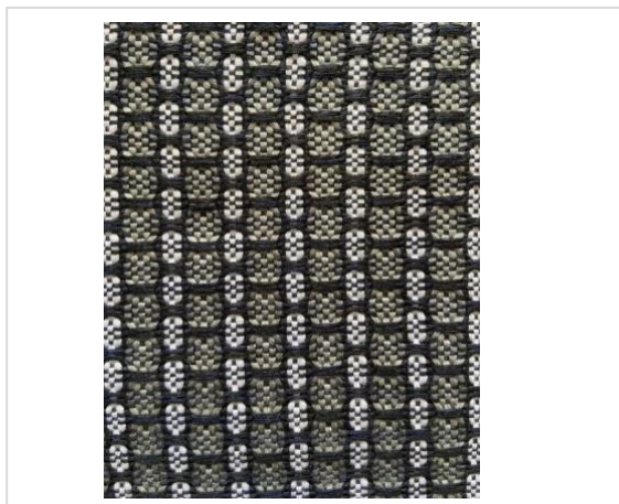
Figure 17: Huck-a-back woven fabric.
