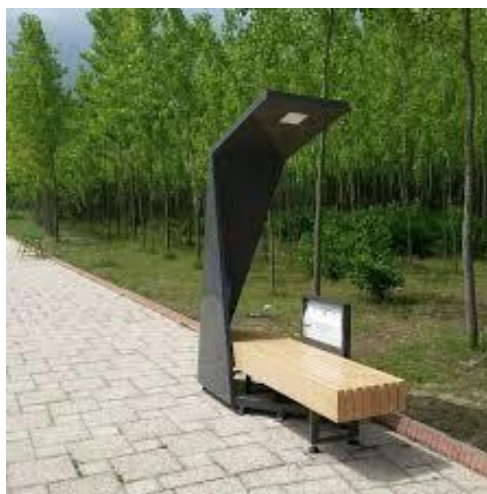
Figure 3: Smart solar bench with the ability to charge electronic devices.
